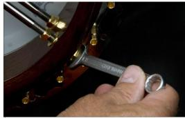
If the action is too high, loosen the nut inside the rim and tighten the outside nut. Strings will go down to the fingerboard.
